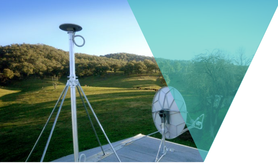
Regional GNSS CORS with satellite communications.
